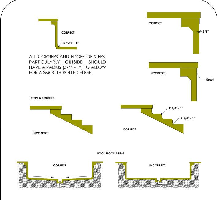
ALL FLAT SURFACES SHOULD HAVE SLOPE TOWARDS THE DEEPEST POINT IN THE POOL. (MINIMUM ½" PER FOOT). THE LOWEST POINT IN THE POOL (TYPICALLY THE MAIN DRAIN) SHOULD HAVE AN AREA DISHED OUT AL LEAST 12"x12"x2".
