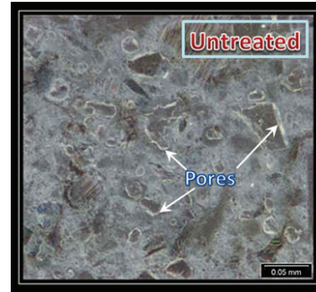
Thin section photomicrographs show reduction in macroporosity and better paste/aggregate bonding after addition of 0.1% Acti-Plex mineral product to the plaster mix.
