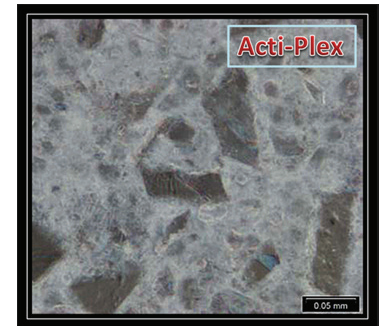
Thin section photomicrographs show reduction in macroporosity and better paste/aggregate bonding after addition of 0.1% Acti-Plex mineral product to the plaster mix.
